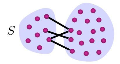
$$\Phi(S) = \frac{\text{\# edges leaving } S}{\text{sum degrees on smaller side, } S \text{ or } V - S}$$
